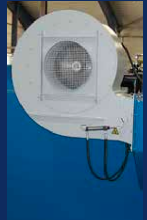
Primary blower - Flue gas fan is not required
