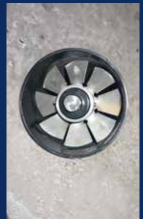
Maintenance-free sludge burner of own design without any moving parts
