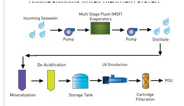
Ultraviolet (UV) light is a form of light that is invisible to the human eye. It occupies the portion of the electromagnetic spectrum between X-rays and visible light. A unique characteristic of UV light is that a specific range of its wavelengths, those between 200 and 300 nanometers (billionths of a meter), are categorized as germicidal – meaning they are capable of inactivating microorganisms, such as bacteria, viruses and protozoa.
