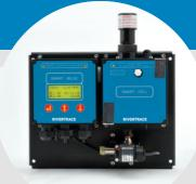
The measuring cell comes as standard with a manual cleaning device for simple routine maintenance to ensure the optical cell is not fouling and maintains accuracy. Alternatively, this can be upgraded to a pneumatic autoclean which will ensure the cell is cleaned at regular intervals without need for manual cleaning.
